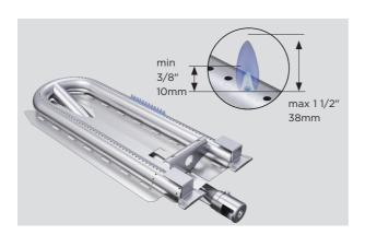
**3.** Flames should be blue and stable. A yellow flame indicates insufficient air. A noisy flame that lifts away from the burner indicates too much air.
