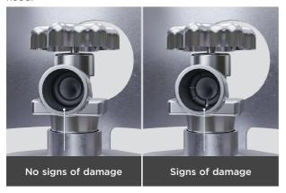
1. Before connecting to the new cylinder, check the rubber O-ring. Do not use new cylinder if O-ring is worn or damaged.
