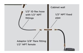
3. If the cylinder is in a separate cabinet, the installer must protect the piping for a distance of at least 2" (50mm) either side of the enclosure opening. An LP cylinder restraint must be installed prior to use (not supplied).
