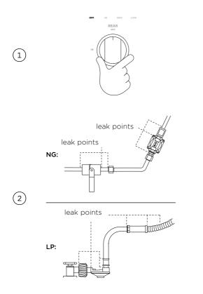
Prepare soap solution by combining one part liquid detergent and one part water. Pour into a spray bottle. Ensure all control valves are in the OFF position before turning the gas supply ON.
