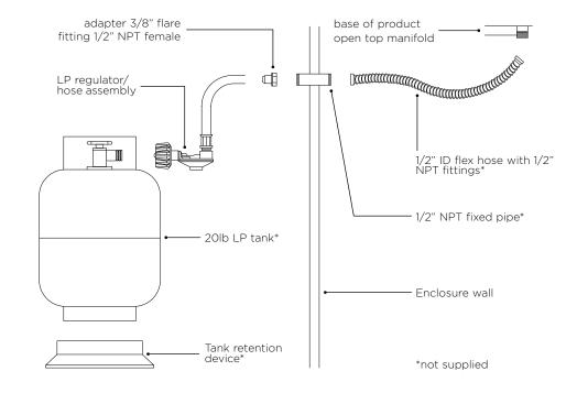
A complete gas tightness check must be performed at the installation site. Periodically check the whole system for leaks, or immediately if the smell of gas is present.
