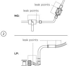
Check all connections from the supply line or LP cylinder by applying the solution around the connection, tubing and end of the manifold. Soap bubbles will appear where a leak is present.
