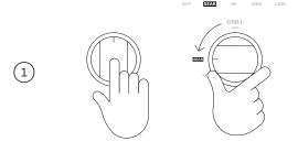
Push in and hold the selected dial for 2 seconds before turning to SEAR. Hold for 10 seconds to light the selected burner.
