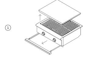
Remove the drip pan and any other removable components from the grill.
