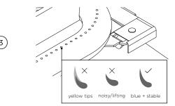
Reinstall the U-burner and light to check. If the flame is blue and stable, remove the burner, tighten the air shutter screw and replace all parts. If flame is still unstable, repeat the above steps.
