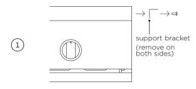
Remove the support brackets from the sides of the grill and replace with the supplied cart mount brackets.
