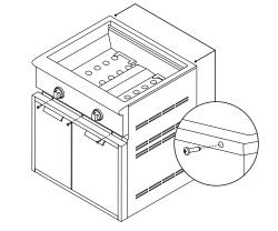
Secure the grill to the cart with two Phillips-head screws at the rear and three at the front.
