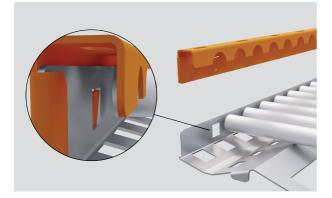
**2.** Lock the rods in place by pushing the side bracket into place.
