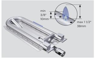
**3.** Flames should be blue and stable. A yellow flame indicates insufficient air. A noisy flame that lifts away from the burner indicates too much air.
