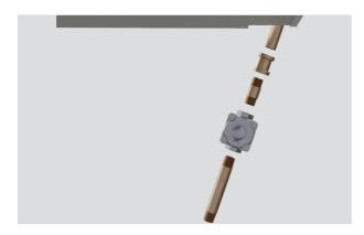
**2.** Ensure that the regulator arrow points in the direction of gas flow away from the gas supply.
