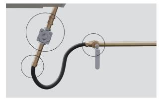
**3.** If a leak is present, immediately turn off the gas supply, tighten any leaking connections and re-check. If you cannot stop a gas leak, turn off the gas supply and call your local gas utility, or the dealer you purchased the appliance from.
