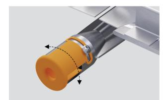
**2.** Using a Phillips screwdriver, loosen the burner shutter screw and turn shutter to desired position.
