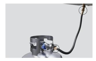
2. Apply a soap solution of 1:1 liquid soap and water to all connections, hoses and fittings from the cylinder to the connection at the grill.
